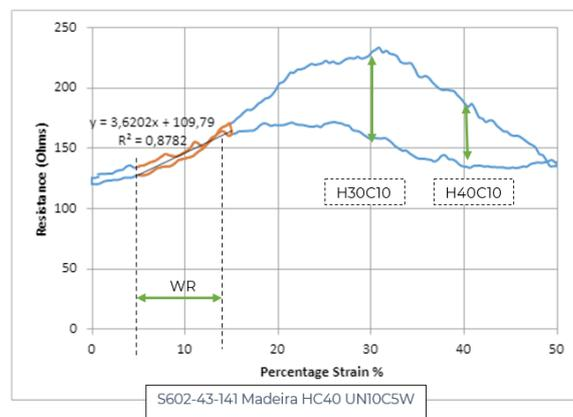
Figure 2 Example of the strain sensor parameters working range (WR), linearity  $R^2$ , hysteresis H30 and HC40 at 30% and 40% strain for the Madeira HC 40 sensor with uncoated threads
