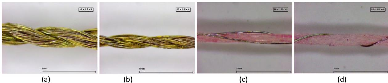
*Figure 4 Examples of coated threads: (a) Madeira HC12, (b) Madeira HC40, (c) Elinox PESHTdtex1402VN35 and (d) Elinox PES280dtexVN35PES20dtex*
