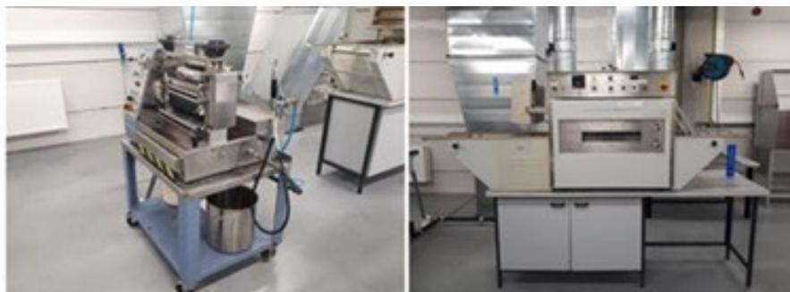
*Figure 3 Pilot line: dip coating and drying unit (Mathis)*
