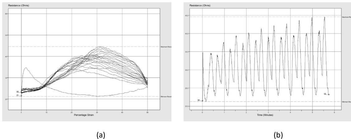
Figure 6 Example of coated MadeiraHC12 sensor after 5 WC: (a) resistance vs. strain and (b) resistance vs time (10 SC)
