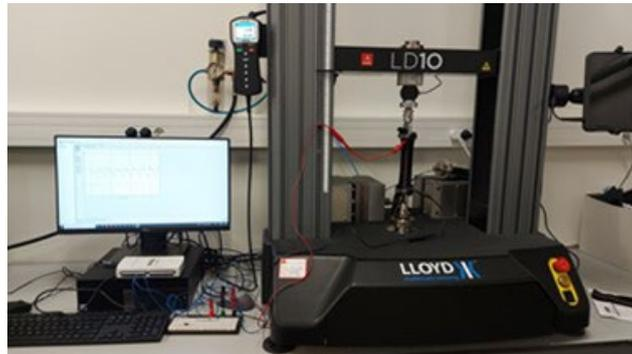
Figure 5 Test set-up: tensile tester and DAQ
