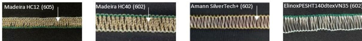
Figure 1 Examples of stitches 605 and 602 (ISO 4915:1981) using various EC-threads as cover thread (close-up stitch front)
