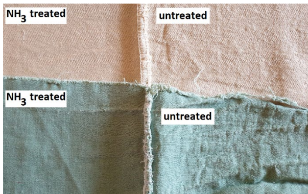
Figure 5: Heavy hemp canvas weave – fabric conservation during washing (60°C) via Beau-Fixe®
