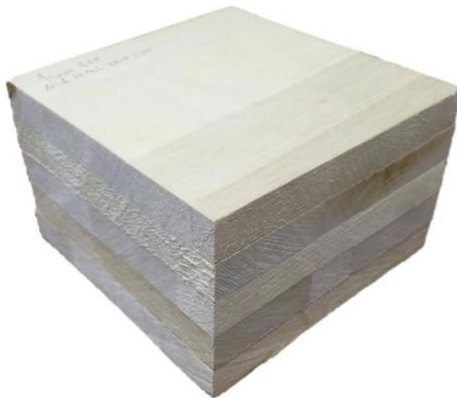
Figuur 25 CLT made from aspen (Populus tremuloides) (Espinoza en Buehlmann, 2018)
